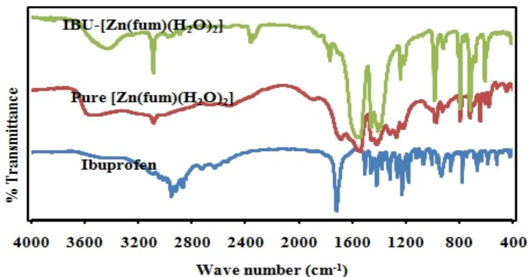
**Figure 2: Infrared spectra of [Zn(fum)(H<sub>2</sub>O)<sub>2</sub>] before and after loading of Ibuprofen**
