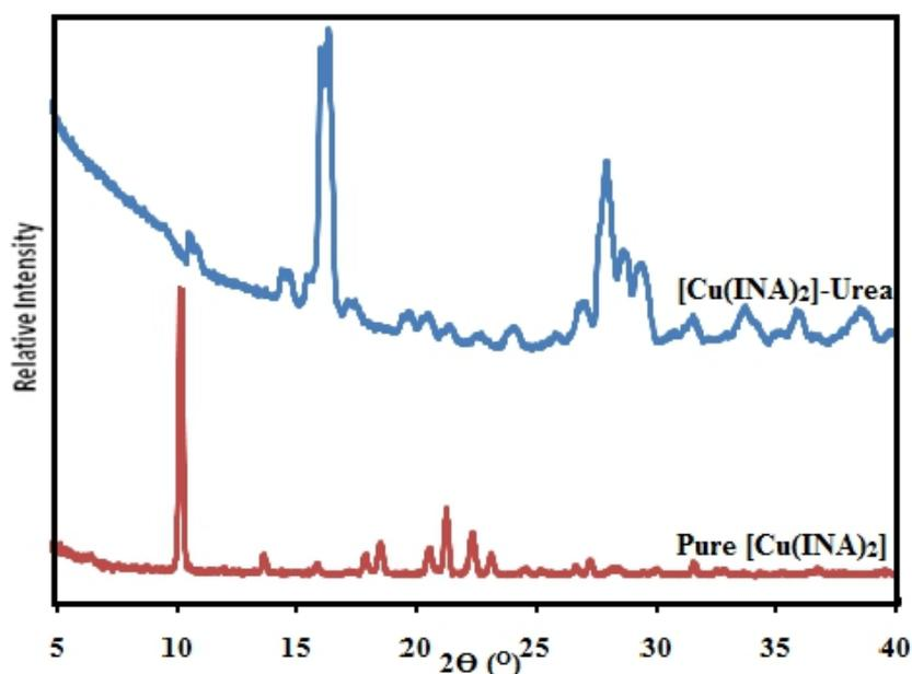
**Figure 7: XRPD of [Cu(INA)<sub>2</sub>].H<sub>2</sub>O before and after loading of Urea**
