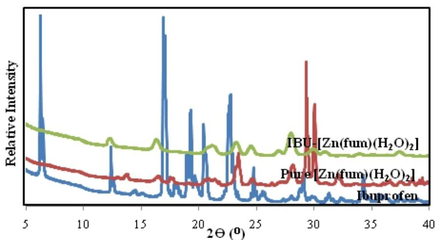
**Figure 3: XRPD of [Zn(fum)(H<sub>2</sub>O)<sub>2</sub>] before and after loading of Ibuprofen**
