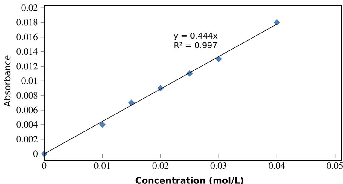
**Figure 1: Calibration Curve obtained from the absorption spectrum in the ultraviolet-visible spectral region for the Ibuprofen solution.**
