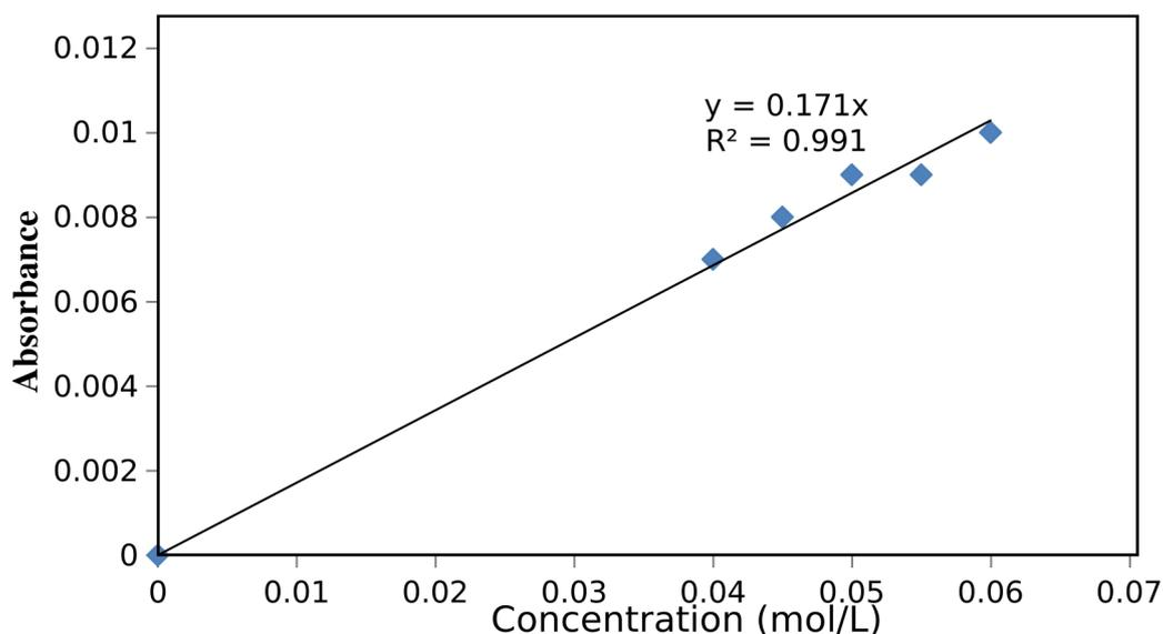
**Figure 5: Calibration Curve obtained from the absorption spectrum in the ultraviolet-visible spectral region for the Urea solution.**
